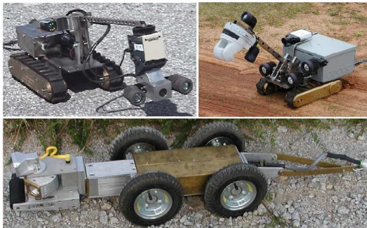
Figure 13. Three ventilation tunnel robotic inspection systems [63]
